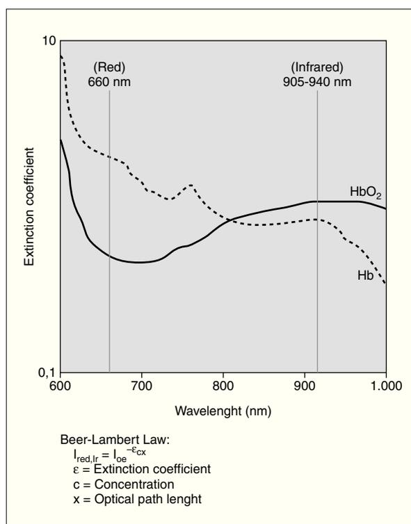
**Figure 1.** Relation between extinction coefficient and wavelength, in nanometers (nm), detecting both red and infra red light, at 600 nm and 905-940 nm.
