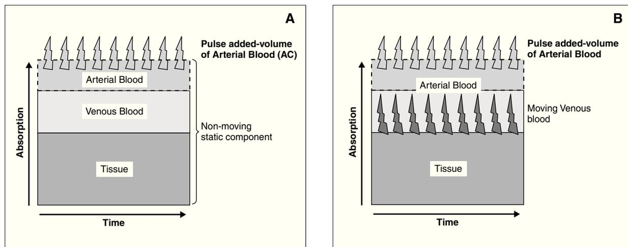
**Figure 2.** A) When light passes through tissues some of the light is absorbed. Without motion, the only variable light absorption is by the arterial blood (AC). B) During motion, conventional  $SpO_2$  displays falsely low value since it measures arterial AND non arterial pulsatile components.
