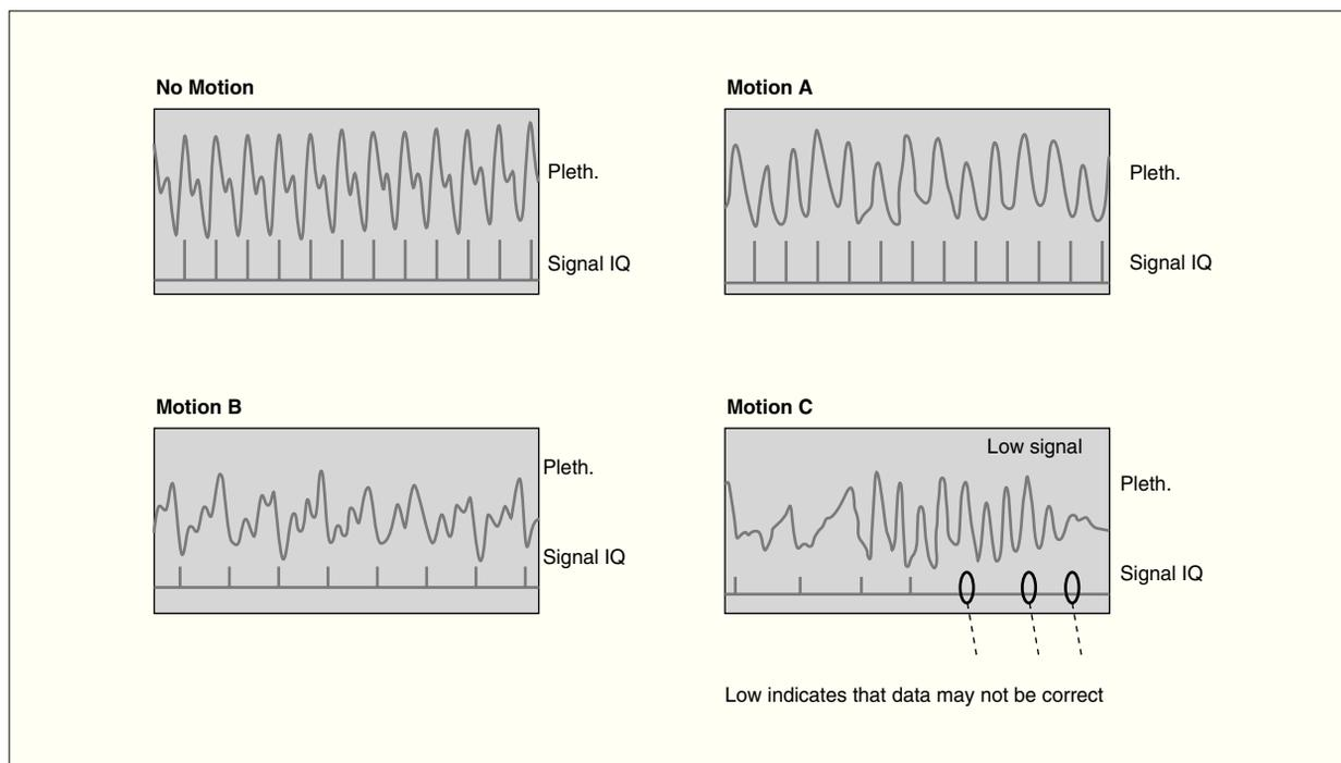
**Figure 6.** Signal IQ which permanently verifies the quality of the signal (see text).
