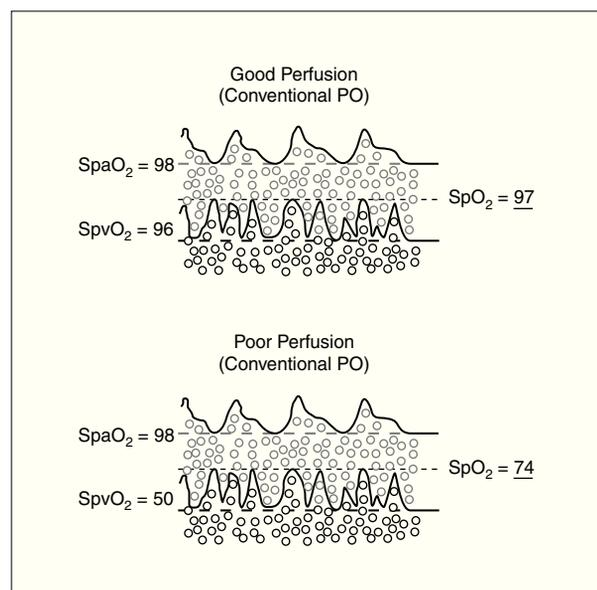
**Figure 3.** Influence of perfusion on the accuracy of conventional pulse oximetry during motion and how a reading will be falsely low when venous saturation is low.
